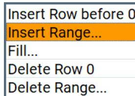
"Insert Range" Insert new rows before the marked row. The number of rows to be inserted can be defined in an entry window.
