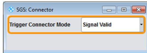
Comprises the settings necessary to configure the signal at the input/output of the multi-purpose "TRIG" connector.
