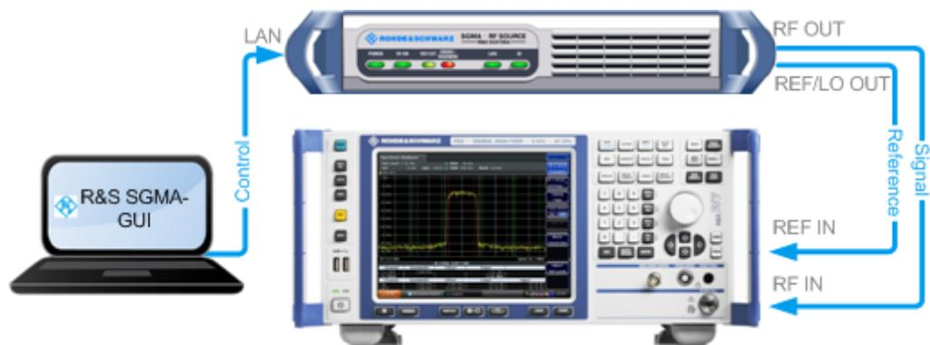
Figure 5-1: Example of the setup
