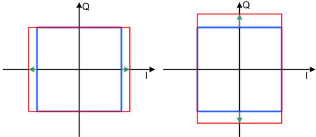
Figure 9-2: Negative gain imbalance (left) and positive (right) gain imbalance in the I/Q constellation diagram
