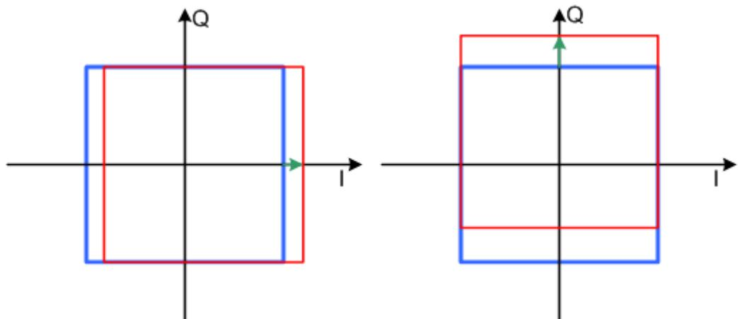
Figure 9-3: I offset (left) and Q offset (right) in the I/Q constellation diagram
